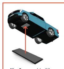
WaveSense consists of the GroundSense sensor, NavSense localization software, and MapSense mapping tool.
